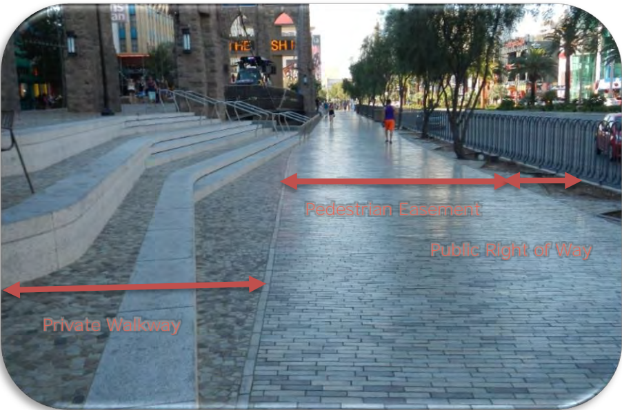
Picture 2.30 – New York-New York Walkway with Public Right-of-way, Pedestrian Easement, and Private Walkway.
